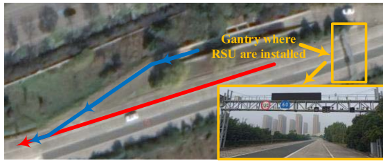
Fig. 3. Test field for V2I data collection.
