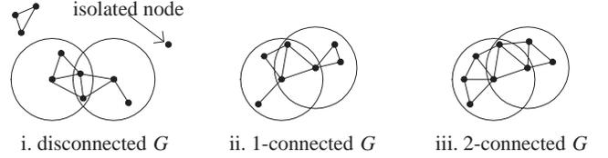
Fig. 3. An illustration of graph  $k$ -connectivity. Note that 1-connectivity has the same meaning as connectivity.
