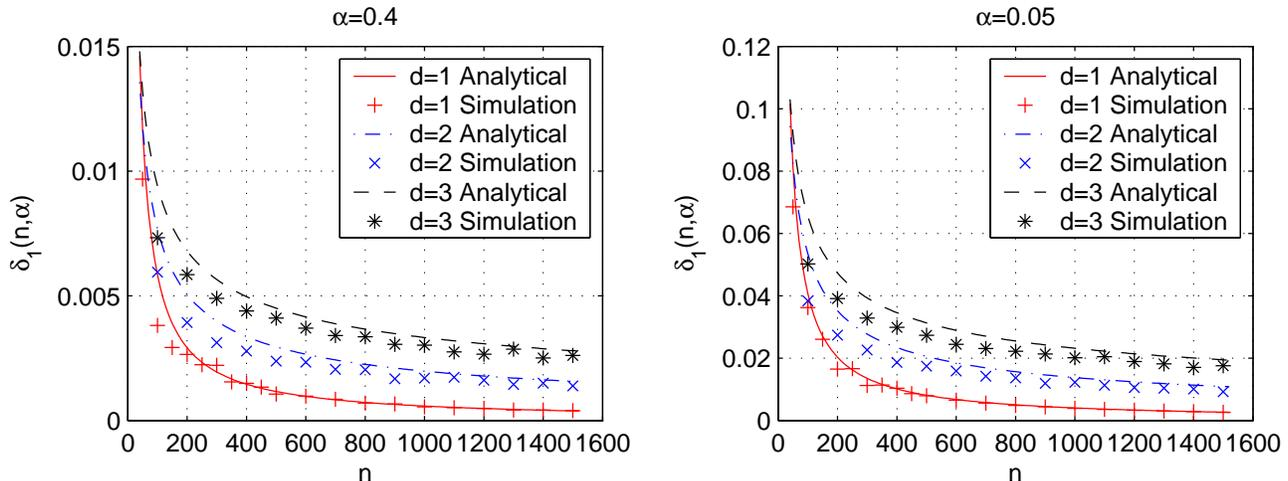
Fig. 10. Phase transition width of 1-connectivity *versus* the number of nodes  $n$  in  $d$ -dimensional space  $d = 1, 2, 3$ . The value of  $\alpha$  is fixed in each scenario. For the analytical results, the boundary effect is ignored; for the simulation results, the boundary effect is eliminated by using the toroidal distance metric.
