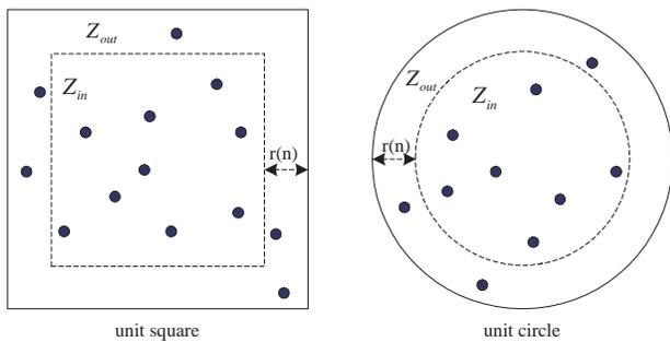
Fig. 9. An illustration of the first method for avoiding the boundary effect in 2-dimensional network area. Only nodes located in subarea  $Z_{in}$  are counted for the statistics in the simulation.
