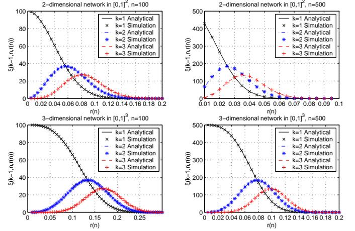
Fig. 5. Expected number of nodes with degree  $k$  ( $k = 1, 2, 3$ ). For the analytical results, the boundary effect is ignored; for the simulation results, the boundary effect is eliminated by using the toroidal distance metric [3].
