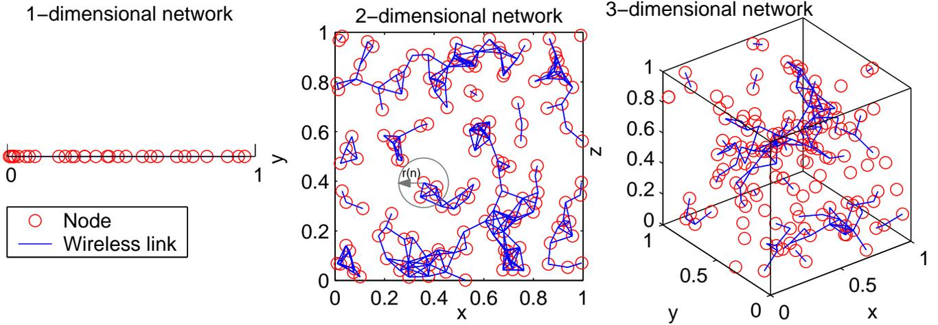
Fig. 2. An illustration of the network model in  $d$ -dimensional space ( $d = 1, 2, 3$ ). A total of  $n$  nodes are randomly and independently distributed in a unit cube  $[0, 1]^d$  following a uniform distribution; each node has a uniform transmission range  $r(n)$ , and any two nodes can communicate with each other iff their Euclidean distance is at most  $r(n)$ .
