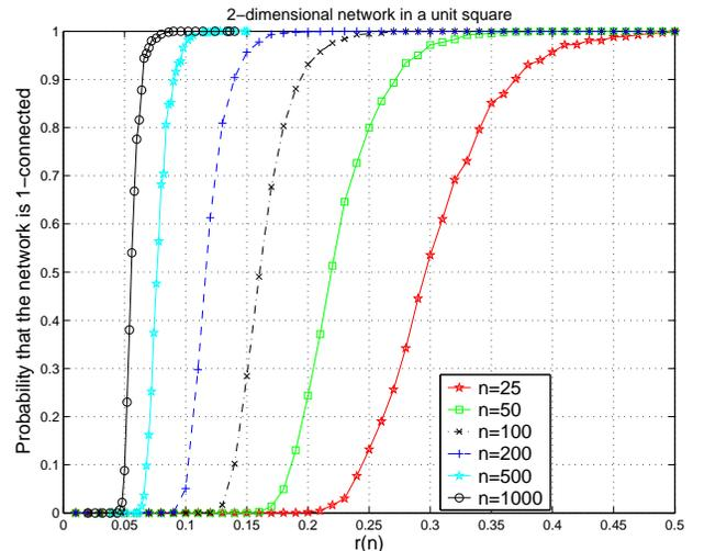
Fig. 1. An illustration of the phase transition behavior of 1-connectivity in 2-dimensional networks through simulations in which a total of  $n$  nodes are randomly and uniformly distributed on a unit square. The probability that the network is 1-connected transits from nearly zero to nearly one over a small range of values of the transmission range  $r(n)$ , and the transition becomes steeper as the number of nodes  $n$  increases.
