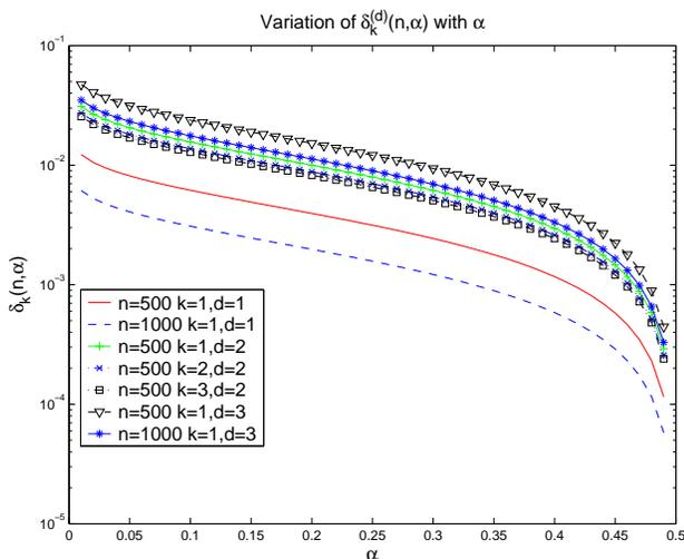
Fig. 8. Analytical results for the phase transition width of  $k$ -connectivity versus  $\alpha$  in  $d$ -dimensional space  $d = 1, 2, 3$ .
