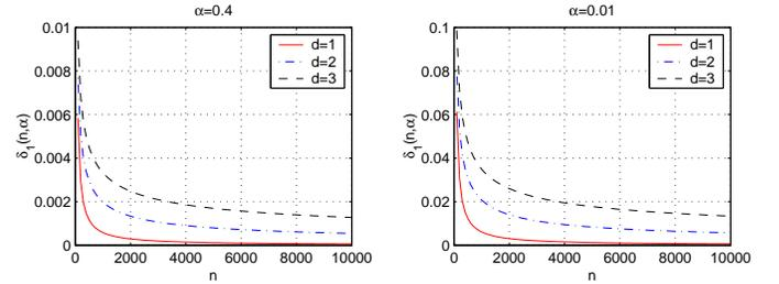
Fig. 7. Analytical results for the phase transition width of 1-connectivity in  $d$ -dimensional space ( $d = 1, 2, 3$ ). The value of  $\alpha$  is fixed in each scenario.
