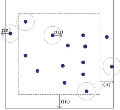
Fig. 4. An illustration of boundary effects in a 2-dimensional network. The nodes located close to the border of the network area have lower average node degree compared with the nodes located in the inner part of the network area.
