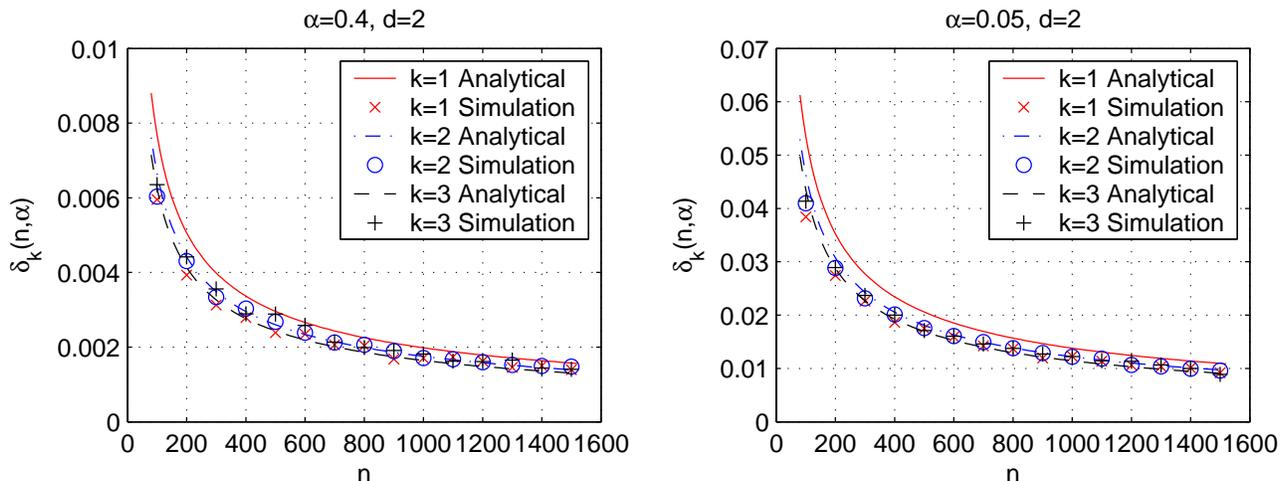
Fig. 11. Phase transition width of  $k$ -connectivity ( $k = 1, 2, 3$ ) *versus* the number of nodes  $n$  in 2-dimensional space. The value of  $\alpha$  is fixed in each scenario. For the analytical results, the boundary effect is ignored; for the simulation results, the boundary effect is eliminated by using the toroidal distance metric.
